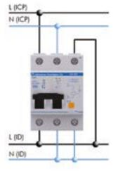
**IGA TEST PLUS** series protectors cut off the power supply when they detect a permanent overvoltage or undervoltage, (for example, a fault in the neutral), thus protecting the equipment installed downstream.
