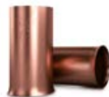
AT-072NCXX: Copper adapter sleeves with variable diameters depending on XX selection. XX indicates the mm 2 of the desired cable. They increase the conductor diameter fitting it in a mould designed for bigger cables. X=50, 70, 120...
