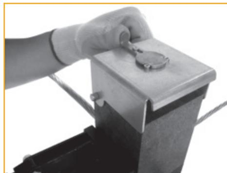
**7. Ignite the Starting Powder using the Spark Lighter AT-060N.**
