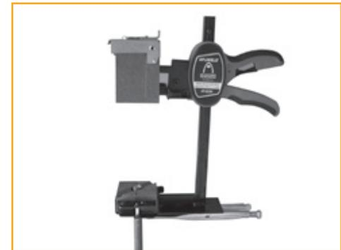
Now the clamp should remain estable on the pliers, letting both hands free to place later the rest of conductors easily
