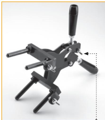
Adjustment wingscrew in AT-049N and AT-050N clamps
